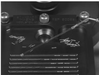
The Seed Alignment Tray connected to the Seed Sterilization and Sorting Tray. A SeedVac™ is picking up the seeds.
