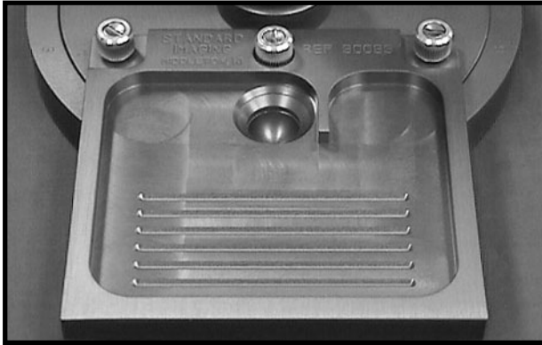
Fig. 1: The Seed Alignment Tray attached to the Loading Cover.
