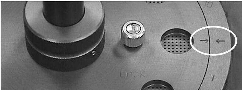
*Fig. 2: The cover in the LOCK position.*
