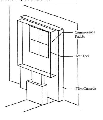
The Digital X-Ray Field Test Tool consists of a copper pattern which provides a ±5cm by ±5cm alignment pattern with 1mm resolution.
