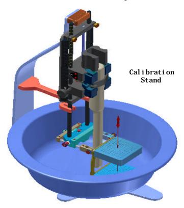
appropriate gauge needle into a central hole coordinate in the grids so that the needle is supported by both grids. Verify on the ultrasound display the coordinate of the needle in the grid. Continue and check alternate co-ordinates around the grid and verify the needle path meets local standards.
