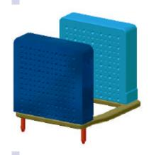
NOTE: The calibration plate is exactly 5 mm (1 row) in thickness.
